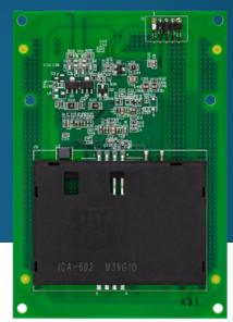
Dual interface USB CCID reader/writer module supports contact ISO/IEC 7816 (ID-1 Slot) contactless ISO/IEC 14443.
